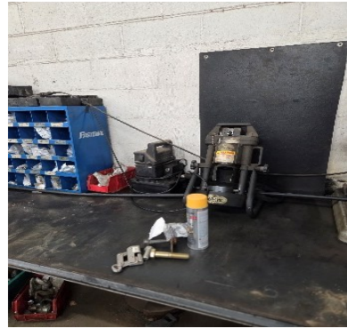
Gates hose crimper & fittings On-site hydraulic hose fabrication — strong margin line.
