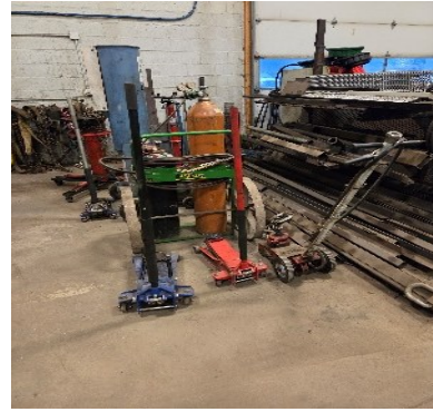
Three floor jacks, 10-ton air jack & torch cart
